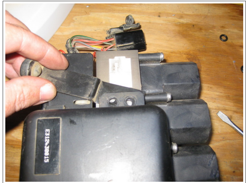
Replace the pressure switch if you removed it. I applied a dab of Loctite thread sealant to keep it sealed.
